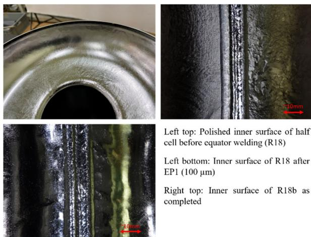
Figure 7: Inner surface of each cavity.
