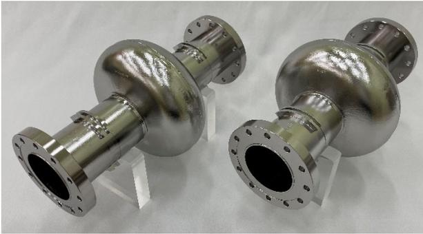
Figure 3: Fabricated cavity (R18 and R18b).
