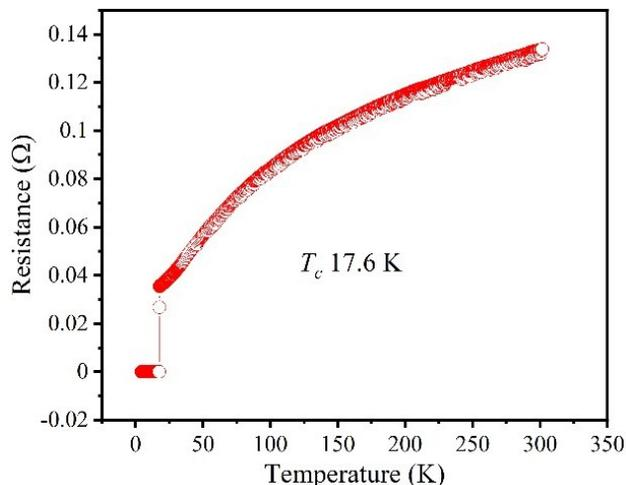
Figure 2: Resistance as a function of temperature of the Nb<sub>3</sub>Sn film fabricated by co-sputtering.
