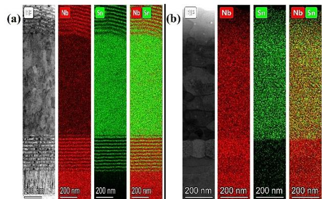
Figure 1: TEM image and EDS mapping of (a) as-deposited Nb-Sn multilayers, and (b) annealed Nb<sub>3</sub>Sn film.
