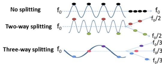
Figure 1: Two-way and three-way equal splitting scheme with deflecting cavities.
