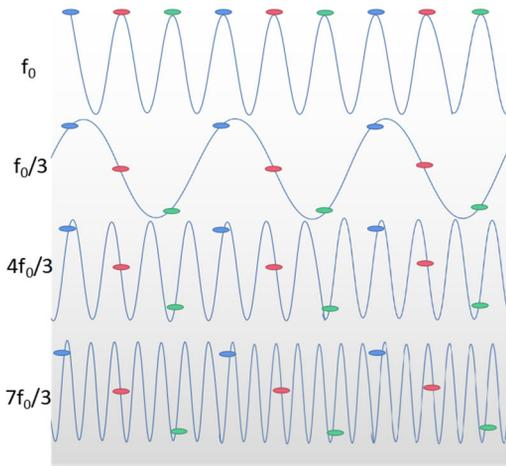
Figure 5: Three-way splitting scheme with RF deflecting cavity frequency equal to  $f_0/3$ ,  $4f_0/3$ ,  $7f_0/3$ .
