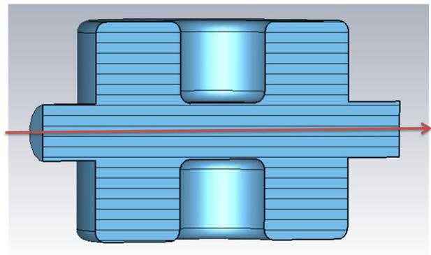
Figure 6: Section view of the double quarter-wavelength cavity with beam axis.
