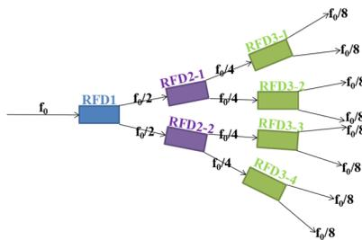
Figure 2: Eight beam lines with seven deflecting cavities classified into three categories.
