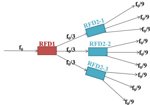
Figure 3: Nine beam lines with four deflecting cavities classified into two categories.
