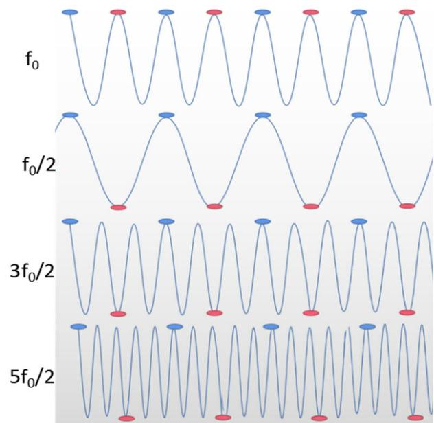
Figure 4: Two-way splitting scheme with RF deflecting cavity frequency equal to  $f_0/2$ ,  $3f_0/2$ ,  $5f_0/2$ .
