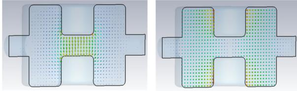
Figure 7: Transverse electric field distribution and magnetic field distribution for a 243.75 MHz double quarter-wavelength deflecting cavity.
