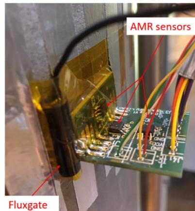
Figure 1: Set of three AMR sensors (X, Y and Z) and fluxgate installed on a cavity.
