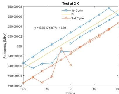
Figure 3: Short step hysteresis of the stepper motor.
