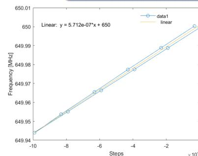
Figure 4: Large step stepper motor hysteresis.
