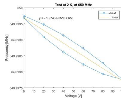
Figure 5: Piezo hysteresis of both capsules with 20 V intervals.
