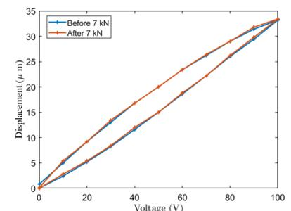
Figure 6: Piezo hysteresis before and after a 7 kN force was applied at room temperature.
